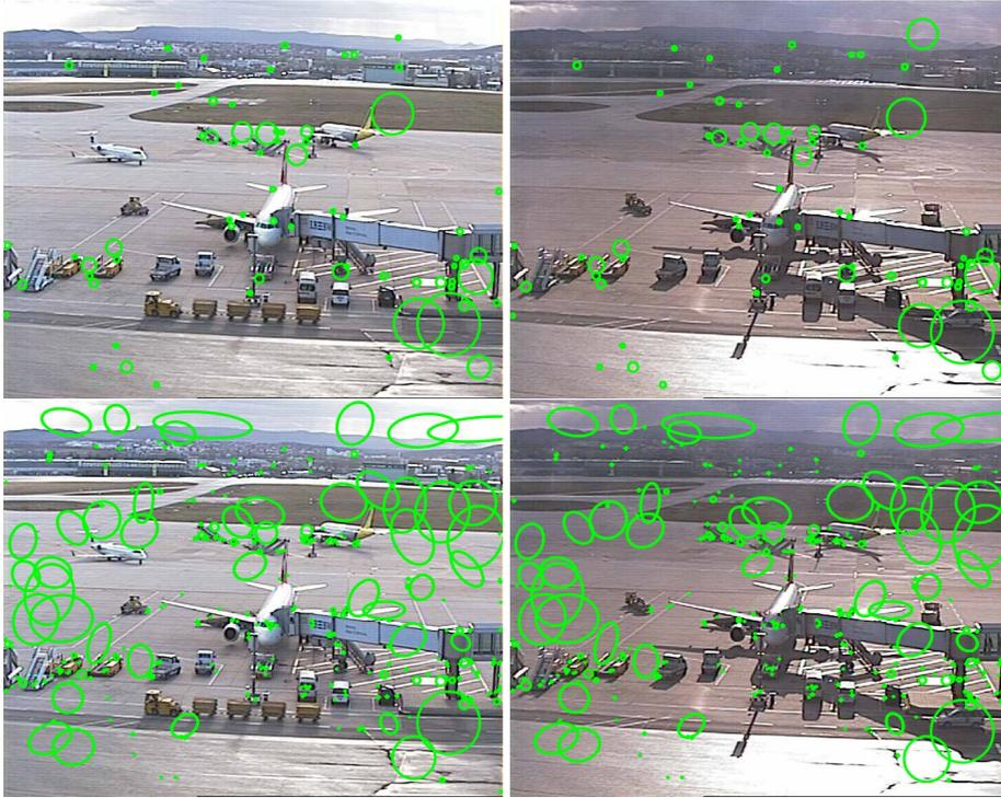
Fig. 5: SIFT correspondences (top), and complementary NF feature [11] correspondences (bottom) between the views in Figures 3(a) and (b) which caused the image-based background model to diverge. From the point-of-view of illumination invariant features, the images are similar since the correspondences cover wide areas.
