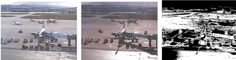
(a) Original view at time  $t_0$ . (b) Illumination changes and reflections at  $t_0 + 10s$ . (c) Foreground from the background model of (b).
