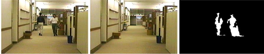
Fig. 2: Background removal using a multivariate background probability. Displayed are input image  $I_t$ , the average background  $\mu$ , and the foreground mask  $F$ . It can be observed, that the shirt of the left person is only partially detected as foreground since it looks similar to the background. Furthermore, shadows on the floor are detected as foreground.
