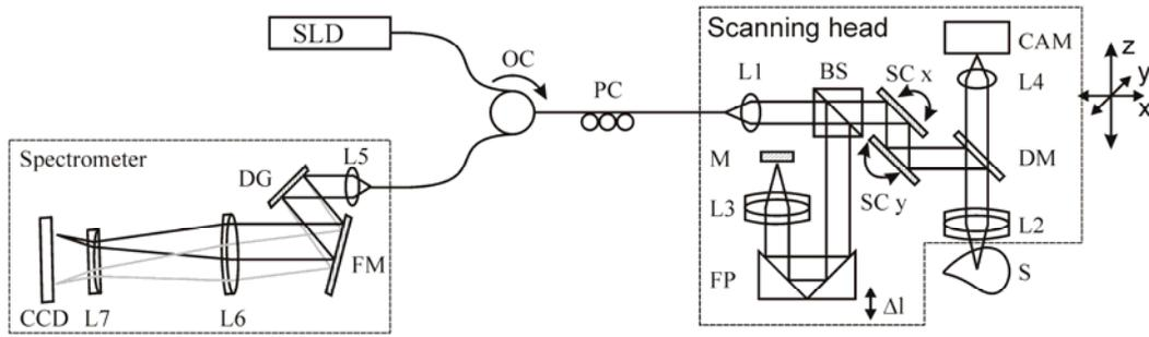
**Figure 1:** Optical setup of the FD-OCT system: SLD - superluminescent diode, OC - optical circulator, PC - polarization controller, L1-L7 - lenses, BS - beam splitter, SC - scanning mirrors, DM - dichroic mirror, S - sample, CAM - video camera, FP - silver coated folding mirrors,  $\Delta l$  - shift reference arm length, M - silver mirror, DG - diffractive grating, FM - folding mirror, CCD - line scan camera.
