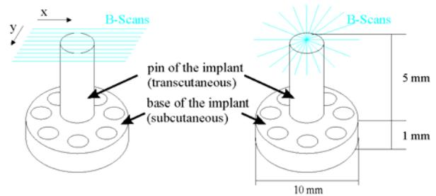
**Figure 2:** Schematic of the percutaneous implant and the scanning scheme for 3D stacks (left) and spoke pattern scans (right).
