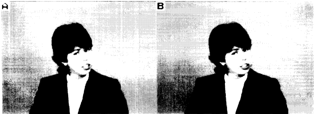
Fig. 15. Coded images of Fig. 11A, data rate: 64 kbit/s. A: block-oriented hybrid coder ( RM8 ); B: object-oriented analysis-synthesis coder ( OBJ.COD. ).
