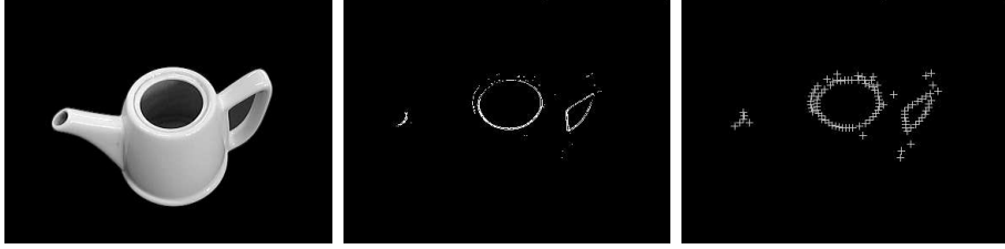
Fig. 8. Image processing steps for getting internal object features: Background subtraction and internal edge detection.
