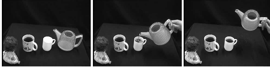
Fig. 12. Example images of the tracked teapot. The hand grasping the teapot leads to outliers during the image silhouette extraction which are detected and eliminated during pose estimation.
