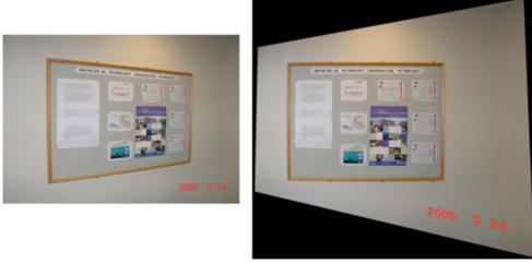
Figure 7: The input image (on the left) is processed by plane homography into the output image (on the right).
