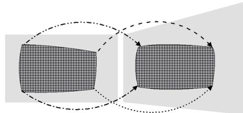
Figure 6: The plane homography transform.
