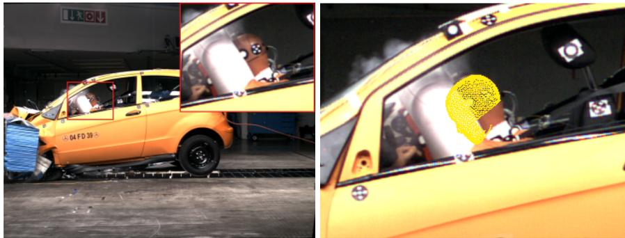
**Fig. 1. Left: a)** Estimating the pose of the dummy’s head from crash test videos is very challenging. The target object is relatively small and partially occluded by the airbag. Furthermore, background clutter and the car’s shadow make it difficult to distinguish the head from the background. **Right: b)** Estimated pose of the dummy’s head. The 3D surface model is projected onto the image.
