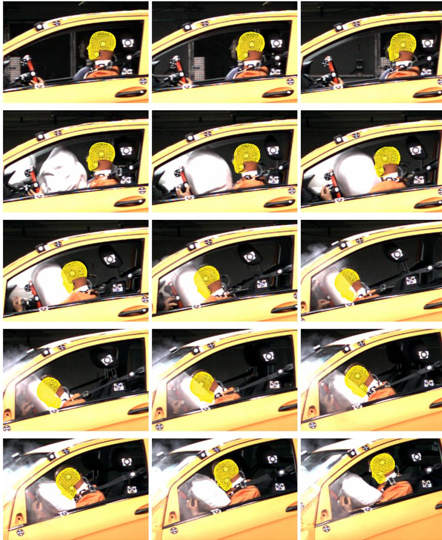
**Fig. 7.** Estimated pose of the dummy's head for frames 7, 22, 37, 52, 67, 82, 97, 112, 127, 142, 157, 172, 187, 202, and 217 (from top left to bottom right).
