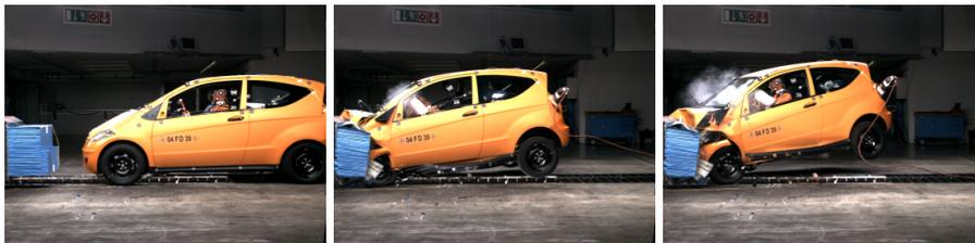
**Fig. 4.** Three frames of the EuroNCAP offset crash sequence. The car jumps and moves laterally due to the offset barrier. The head is occluded by more than 50% at the moment of the deepest airbag penetration.
