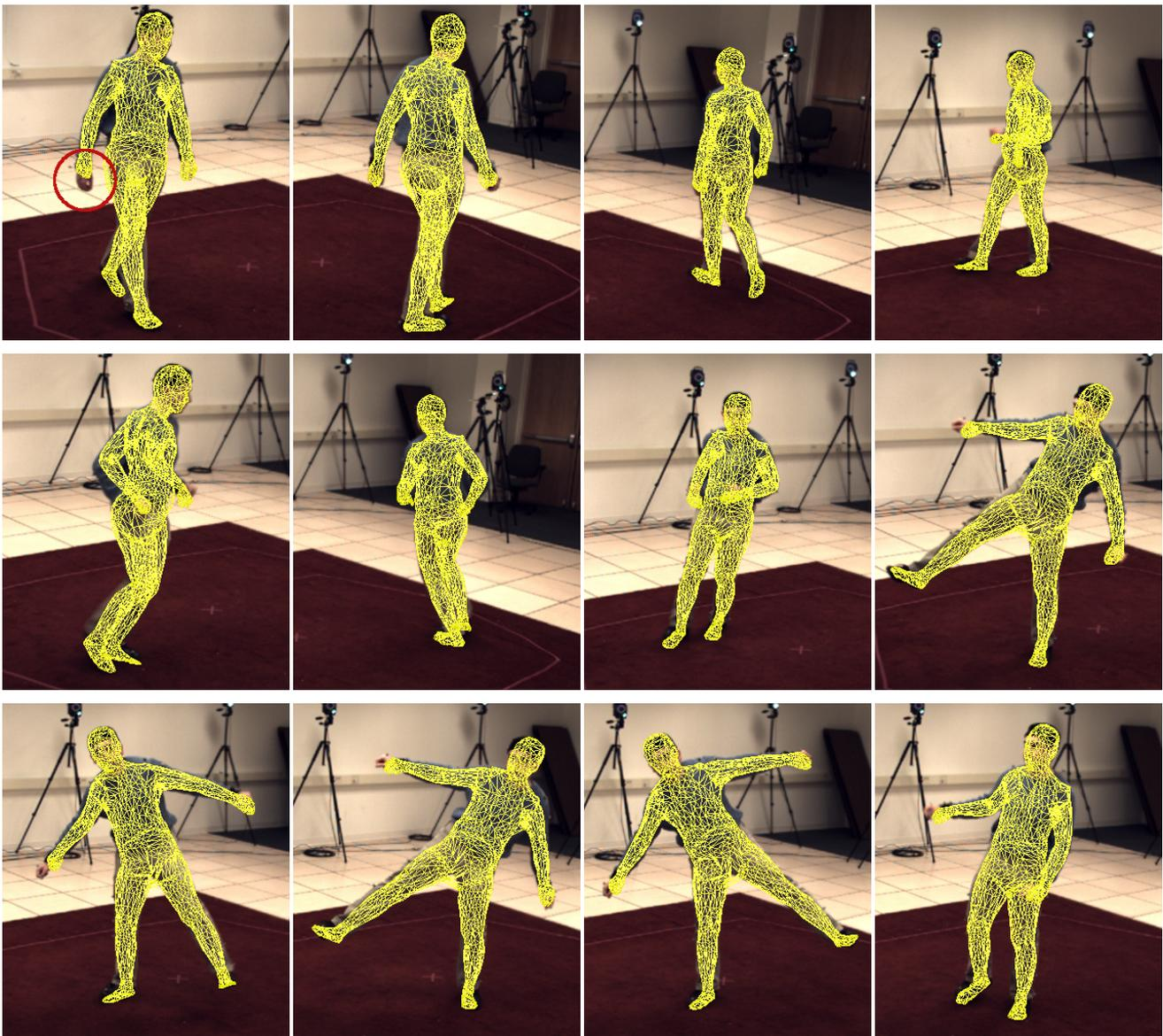
**Fig. 19** Estimates for subject S2. Note that the arms of the surface mesh model are too short, since the model of subject S4 has been used for tracking (*top left*). **From top left to bottom right:** The meshes of the estimates are projected on the images of camera C1 for frames 100, 200, 300, 400, 500, 600, 700, 800, 900, 1000, 1100, and 1200.
