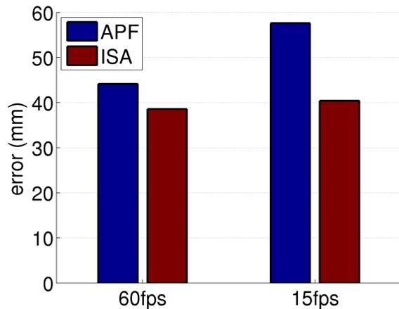
**Fig. 13** The effect of a very fast movement is simulated by using only every 4th frame of sequence S4 (frames 2 – 821). This corresponds to a walking and running sequence recorded with 15 fps. While the error increases slightly by 4.68% to 40.39mm for ISA, the error for APF rises to 57.63mm by 30.5%.
