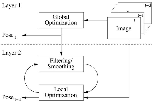
**Fig. 1** A multi-layer framework for tracking. While the first layer based on global stochastic optimization provides robust and relatively accurate estimates, the second layer increases the accuracy and reduces jitter and potential bias from the first layer with a short delay  $d$ .
