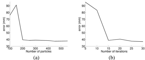
**Fig. 14** Absolute tracking error of global optimization for frames 2 – 821 of sequence S4. Large numbers of iterations and particles improve the estimates only marginally. **From left to right:** a) Error with respect to the number of particles using 15 iterations. b) Error with respect to the number of iterations using 250 particles.
