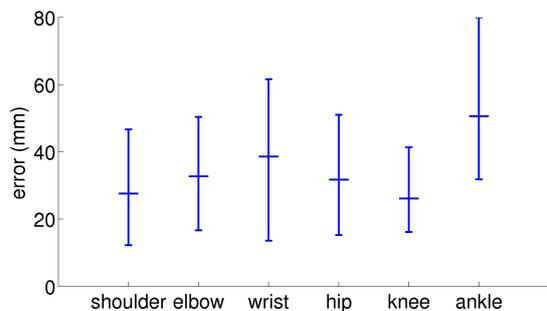
**Fig. 17** Average errors and 0.025-quantiles for individual joints obtained by the multi-layer framework on the entire sequence S4. While the knees are very well estimated, the error bars for the limb extremities such as wrists and ankles are larger than for other joints. The quantiles of the ankles indicate that the ankle joints are not well registered.
