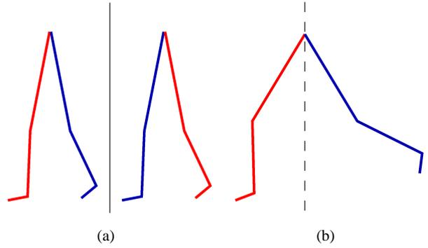
**Fig. 4** Two mutation operators. **From left to right:** *a)* The left branch (red) and the right branch (blue) are swapped. *b)* The left branch (red) is reconstructed from the right branch (blue) by mirroring the first joint.
