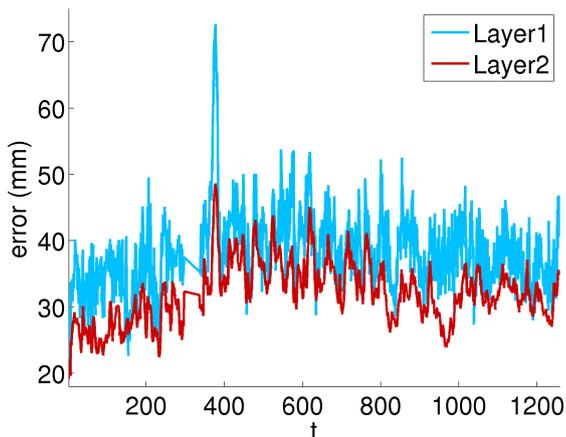
**Fig. 15** Absolute tracking error for the sequence S4 (frames 2 – 1258). The second layer reduces jitter and increases the accuracy of the estimates from the first layer. In particular, the largest error around frame 380 is significantly reduced by the second layer.
