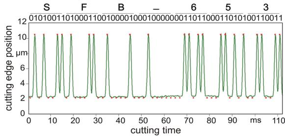
Fig. 4: Example for a signal written as a groove onto the surface.
