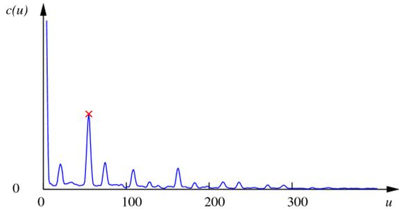
Fig. 7: Amplitude  $c$  of frequency components  $u$  of Fig. 5 in vertical direction. The peak at  $u=54$  corresponds to a groove distance of 14.2 px.
