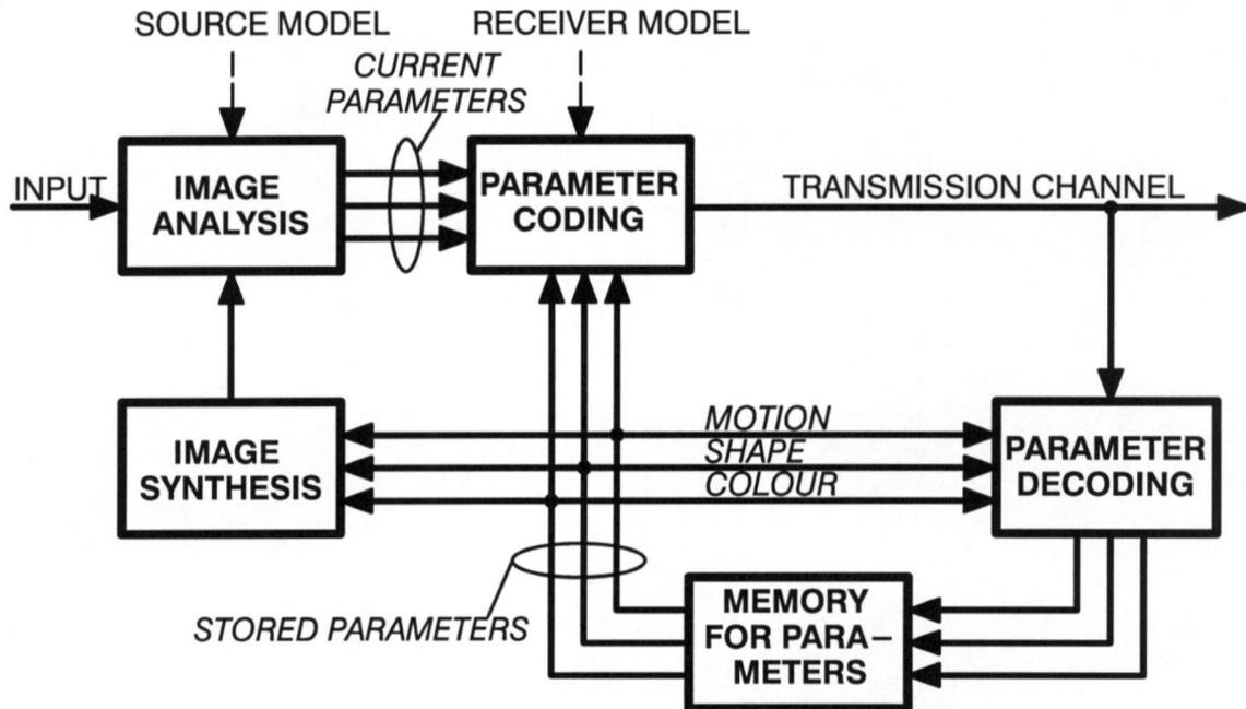
Fig. 2.1: Block diagram of SIMOC.
