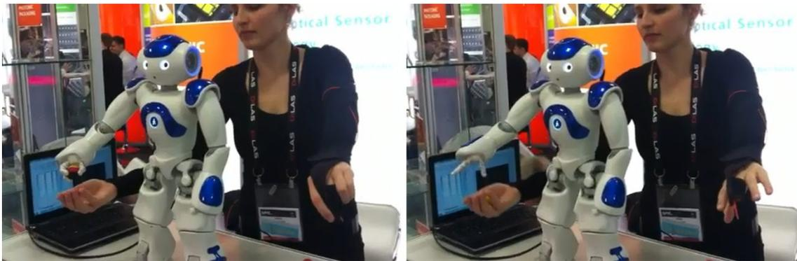
Figure 7. Fiber optically controlled robot with the robot's right arm being steered by a test person's left arm
