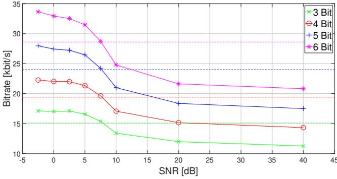
Fig. 4. Mean bitrate across signal-to-noise ratio (SNR) of the lossless codec on the test set. A considerable increase in bitrate with decreasing SNR was observed. The cause is more subbands that are selected at low SNRs. The dashed lines indicate the mean bitrate across the test set. These results were obtained using the complete set of contexts given in Table II.
