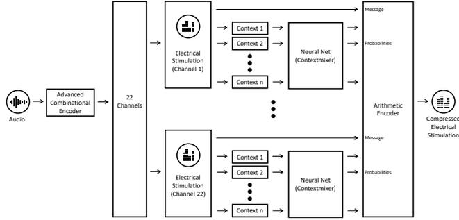
Fig. 2. General structure of the lossless codec. From an audio input the electrical stimulation patterns are generated by the advanced combinational encoder sound coding strategy. A feedforward neural network mixes the estimated probabilities of several contexts to compute (hopefully) improved symbol probabilities which are then used for the encoding of each subband symbol by the arithmetic encoder. The decoder uses the same structure.
