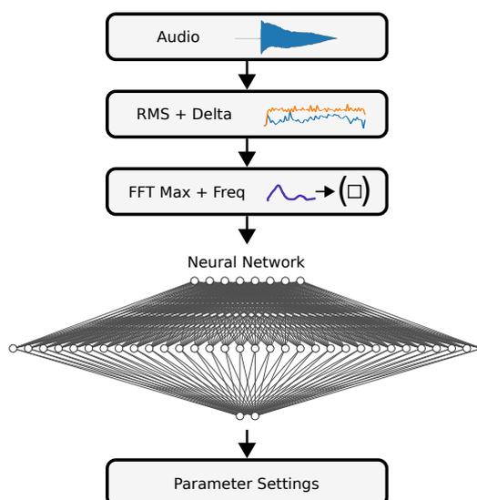
Figure 5: Pipeline for estimation of the three parameters of the tremolo effect
