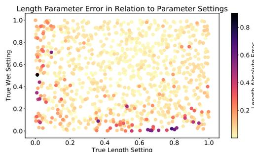
Figure 9: Absolute error of the length parameter estimation plotted against the ground truth setting of length and wet
