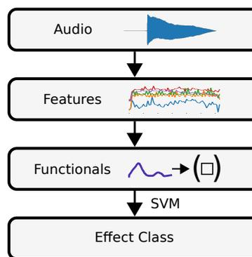
Figure 2: Processing pipeline for recognizing guitar effects
