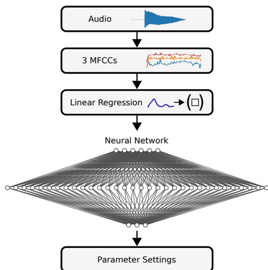
Figure 3: Pipeline for the estimation of the three parameters of the distortion effect
