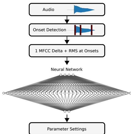
Figure 4: Pipeline for estimation of the three parameters of the delay effect
