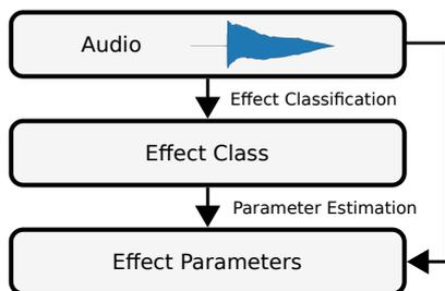
Figure 1: Pipeline for determining the guitar effect and its settings
