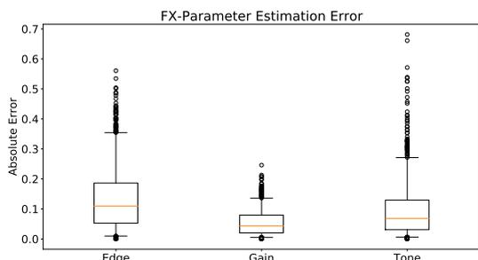
Figure 6: Absolute error of the estimation of the distortion effect parameters: the median is marked by an orange line, the surrounding box covers data from the 25% quartile to the 75% quartile. The whiskers cover the 5th percentile to the 95th percentile; everything outside of those percentiles is an outlier, displayed as circle.
