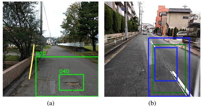
Figure 4: (a) Some damages are difficult to annotate, e.g. when different classes overlap. (b) Rectangular bounding boxes may be a suboptimal choice for some classes, as small ambiguities lead to large variances in IoU.
