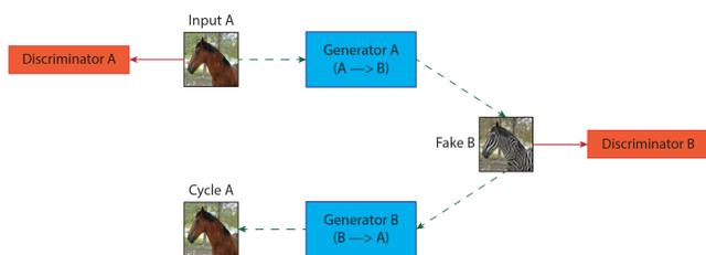
Figure 6: Schematic structure of a CycleGAN. Generator A gets an image from domain A as input and generates a fake image in domain B. Generator B does the same the other way around. The discriminators detect whether an image is real or fake in the respective domain.
