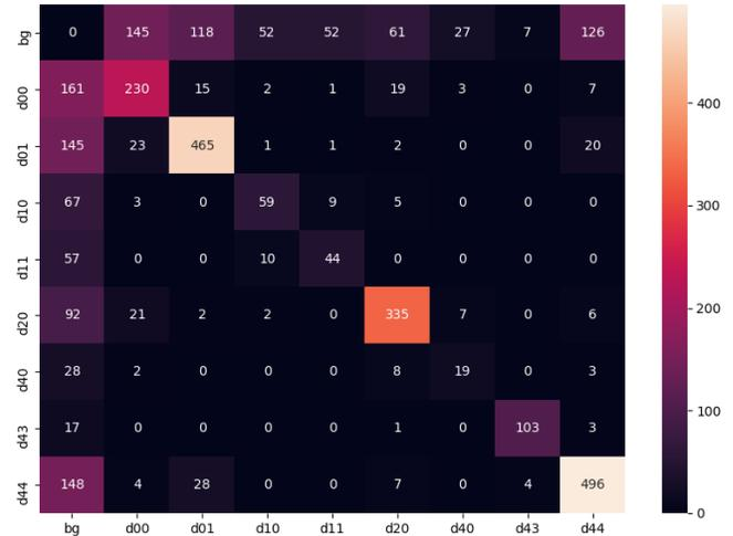
Figure 3: Confusion matrix for all damage classes. Every row corresponds to a detected class and every column contains the ground truth label. *bg* is the background class, i.e. an undamaged road or other objects.
