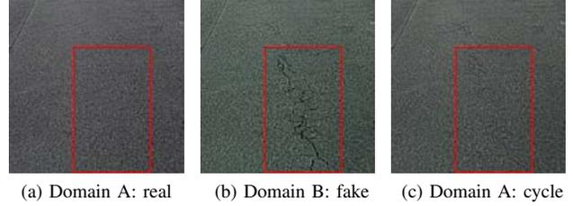
Figure 8: Example for Cycle A of the CycleGAN. Input image (a) without a damage is transformed into an image with road damage (b) which is then removed again (c).
