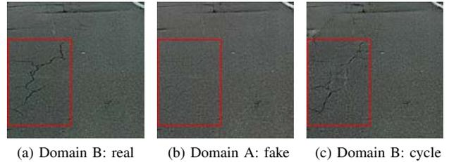
Figure 9: Example for Cycle B of the CycleGAN. Input image (a) with a damage is transformed into an image without a damage (b) which is then added again (c).
