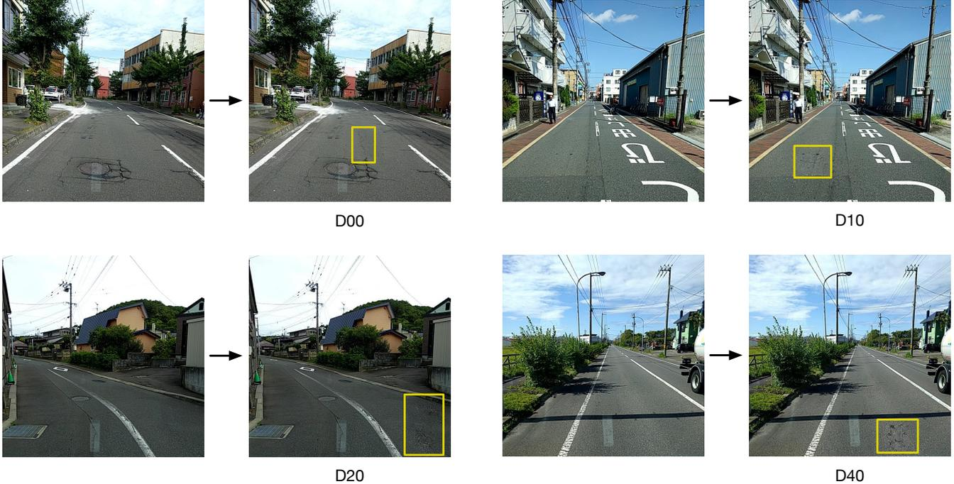
Figure 10: Generating new road damages for training in areas without a damage. Each image pair shows the original image on the left side and the image with a generated road damage (highlighted in yellow) on the right side. Existing bounding boxes are not shown.
