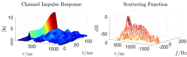
Fig. 6: Illustration of channel impulse responses and the scattering function of the channel corresponding to M-3
