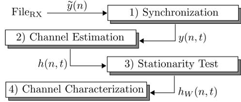
Fig. 4: Data post-processing at the sounder receiver
