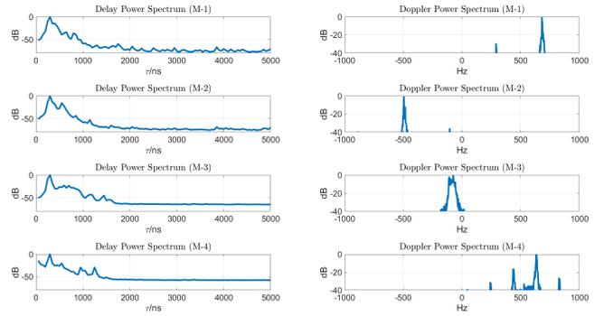
Fig. 7: Delay power spectrum and Doppler power spectrum for  $\{M-i\}_{i=1}^4$
