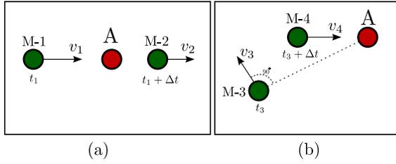
Fig. 5: Illustration of the measurement points  $\{M-i\}_{i=1}^4$  and its velocity vector  $\{v_i\}_{i=1}^4$  with respect to the Receiver-A,  $\Delta t$  is less than 5 seconds.
