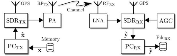
Fig. 1: Channel sounder system block diagram
