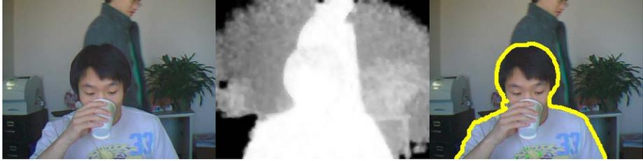
**Fig. 1.** Example segmentation result by fusing color and depth information using Dempster’s theory of evidence. The explicit modeling of uncertainty forces the algorithm to segment the person in the foreground even if the depth information of the person in the background is similar. Input data taken from [9].
