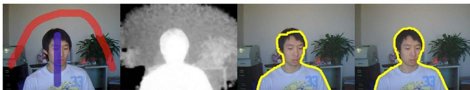
**Fig. 3.** Example interactive segmentation result. From left to right: Color image with initialization (FG in blue/BG in red), corresponding depth image, segmentation result using ToFCut with equal weights, proposed DS fusion with equal weights.
