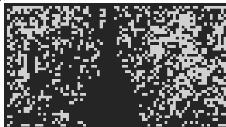
Fig. 4 Assigned macroblock modes for the example in Fig. 3 bottom, grey: LT-GMC, black: other modes
