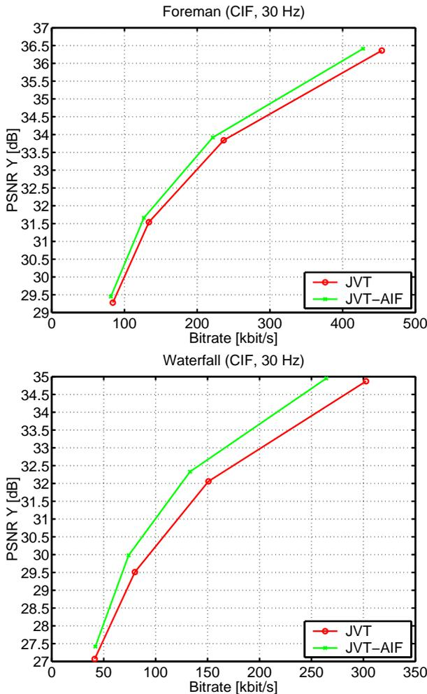
**Fig. 4.** Operational rate distortion curves for test-sequences *Foreman* and *Waterfall*.
