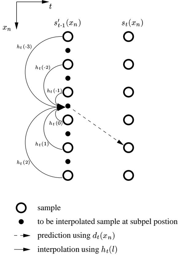
**Fig. 2.** Illustration of motion compensated prediction for a fractional-pel displacement using an adaptive interpolation filter  $h_t(l)$ . Corresponding lines of two consecutive images are shown: The reconstructed reference image  $s'_{t-1}(x_n)$  and the image to be predicted  $s_t(x_n)$ .
