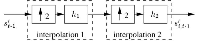
**Fig. 3.** Interpolation process for 1/4-pel displacement vector resolution that is used in the JVT coding scheme. It is based on two steps with two interpolation filters  $h_1$  and  $h_2$ .
