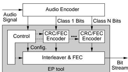
Fig. 4: Block diagram of an Encoder with Unequal Error Protection (UEP) using the EP tool (from [2]).
