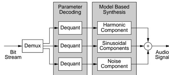
Fig. 3: Block diagram of the HILN parametric audio decoder.
