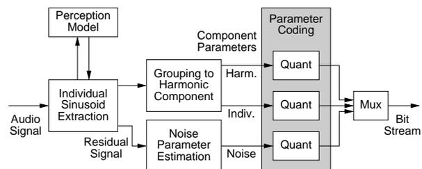
Fig. 1: Block diagram of an HILN parametric audio encoder.
