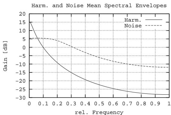
Fig. 2: “Default” low-pass spectra for mean LARs of harmonic and noise components.
