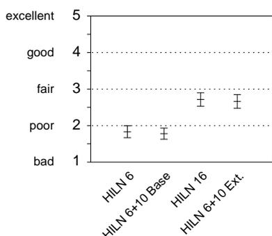
Fig. 5: MPEG-4 Version 2 verification test results for HILN at 6 and 16 kbit/s showing overall mean grading and 95% confidence interval for 7 items and 16 listeners (from [16]).
