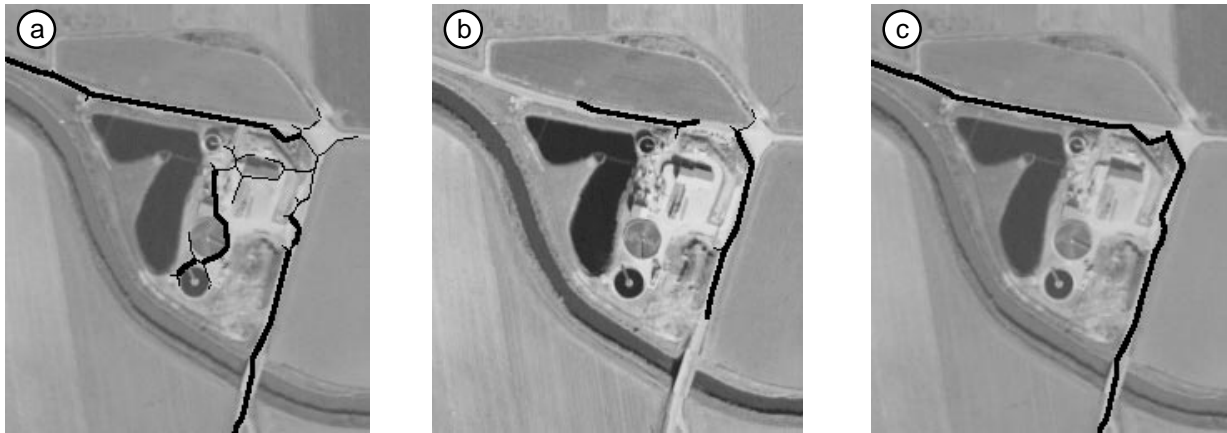
Figure 3. Sensor Fusion demonstrated on the aerial view of a purification plant: Rejected (thin lines) and accepted (wide lines) road features from (a) optical and (b) infrared image with (c) fusion result.
