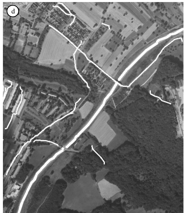
Fig. 8: Segmented (thin lines) and accepted road candidates (wide lines) in (a) SAR image and (b) the corresponding aerial image. (c) Used GIS data for the object class Road and (d) fusion result. The major road is emphasized.
