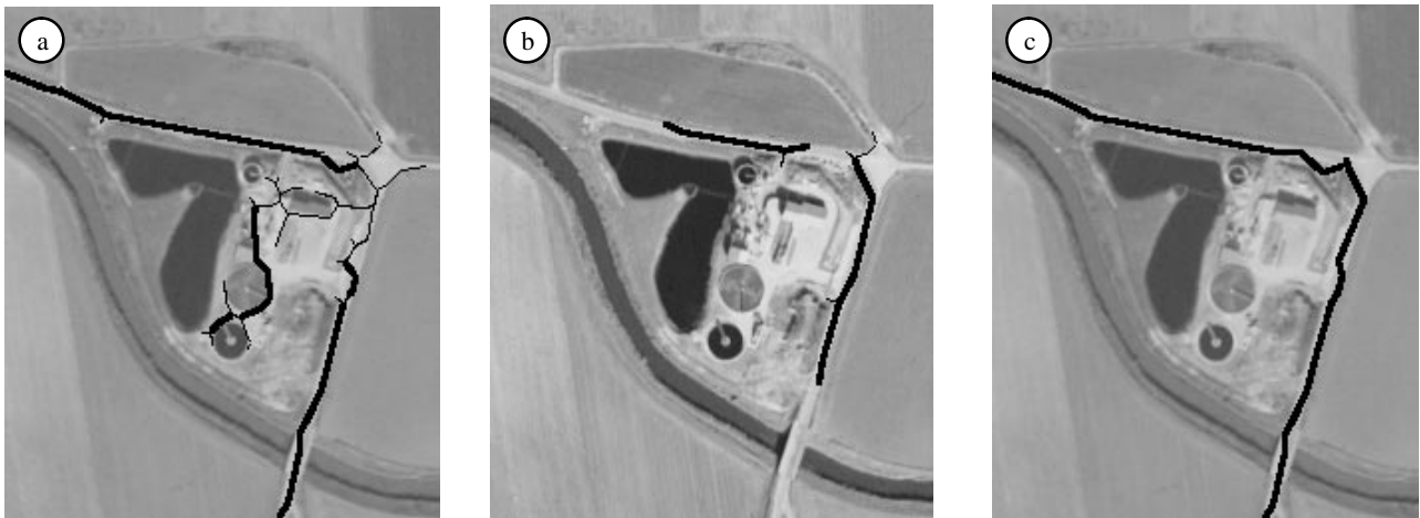
Fig. 7: Rejected (thin lines) and accepted (wide lines) road features from (a) visual and (b) infrared image with (c) fusion result.
