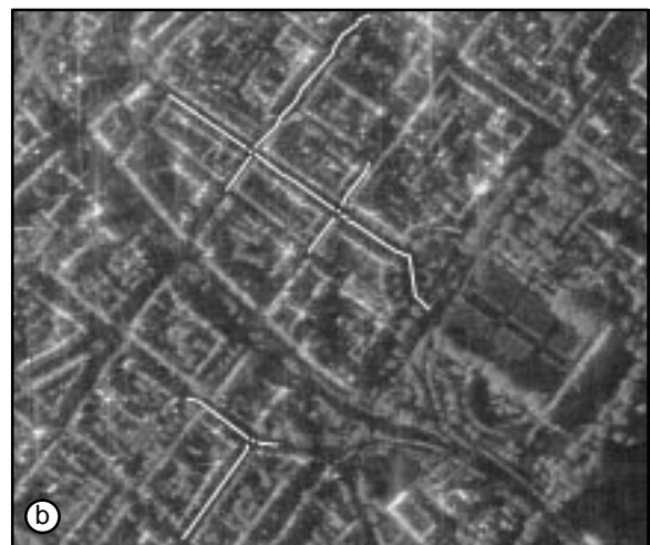
Figure 3: (a) Segmented roads and (b) selected crossroads with interpolated control points in a SAR image
