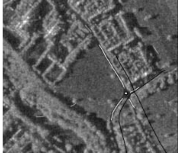
Fig. 4: Expected (black), segmented (grey) and selected roads (white) in the corresponding SAR-image block
