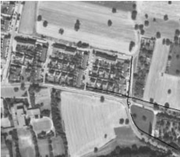
Fig. 3: Expected (black), segmented (grey) and selected (white) roads with computed control point in an aerial image block
