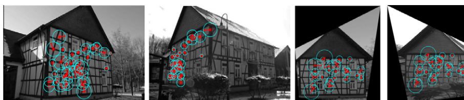
Fig. 9. A number of matched features are shown. Left: on the original images. Right: on the front parallel views. Their scales and orientations are annotated. The feature matches on the viewpoint normalized views have very similar orientations and consistent scale ratios.
