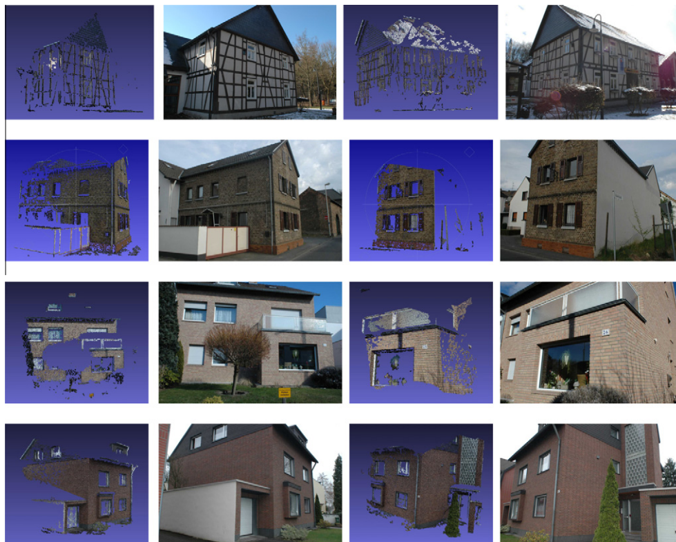
Fig. 5. Four pairs of 3D point clouds and their associated images captured at widely separated views.
