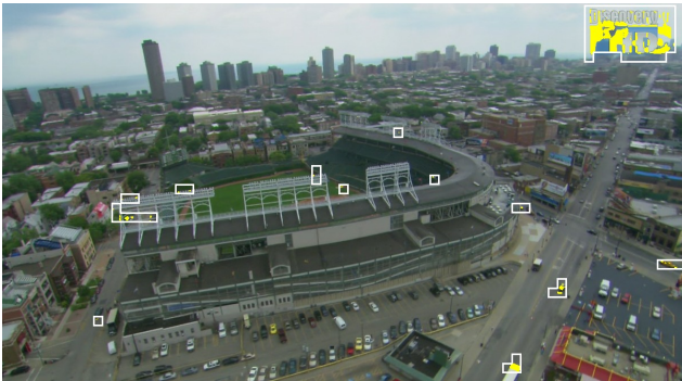
Figure 9. Moving object detection by proposed system. Motion candidate pixel in yellow, moving areas outlined white.
