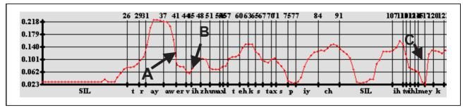
Figure 5. Mouth height as a function of time for the sentence: "Try our Visual Text-to-Speech, it will make ..."; The arrows show where the automatic quality evaluation flagged errors: A: closure too fast; B: missed closure; C: opening too fast. The average contiguous segment length is 6.05 frames with a variance of 2.4 frames, a value judged as good (main influence on 'smoothness').
