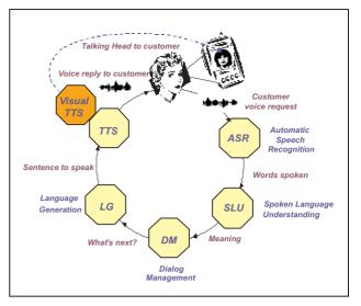
Figure 1. Diagram of any voice-enabled service, extended by Visual Text-to-Speech (VTTS).
