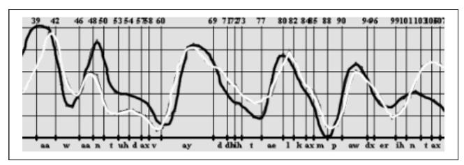
Figure 3. Mouth height as a function of time for the sentence: "I want to divide the talcum powder into ...". The black line shows the recorded values, the white one the values of the synthesized articulation. For a quality score of 'precision', the differences in mouth height between recorded and synthetic samples are summed and normalized by the number of frames.
