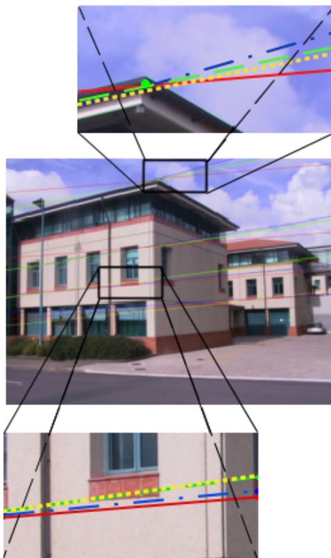
Figure 6: Epipolar lines result from different data sets: green (dashed) lines from data without generated noise, the red (straight) lines from noisy data, the blue (dash-dotted) lines or yellow (dotted) lines from noisy data and the use of collinearity or coplanarity knowledge, respectively.
