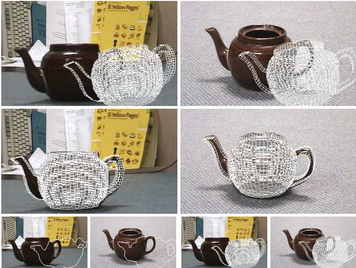
Figure 18: Top row: Stereo image with a teapot. The initialization is quite far away from the object. Center row: Result in the steady state. The coupled contour extraction and pose estimation move the object prior into the right pose. Bottom row: Contour and pose with a simple concatenation of segmentation and pose estimation, i.e., only one iteration. The contour is restricted to the initial, bad pose and cannot fully capture the object. Consequently, the pose stays very close to the initialization.
