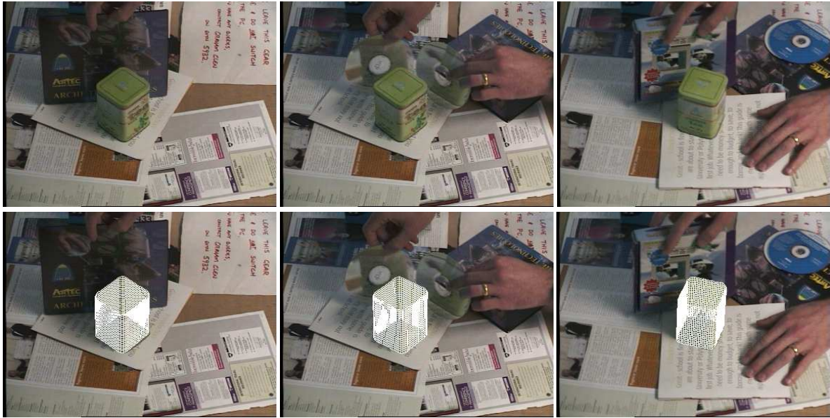
Figure 13: Top row: Input images for frames 51, 189 and 450 of an image sequence containing 560 frames. Bottom row: Pose results. The algorithm is able to deal with a cluttered and changing background.
