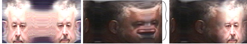
Fig. 5. Texture fusion: The images from the stereo setup are merged to get a texture map for the head: the left texture gives a good face, whereas the right texture gives a good ear and side view of the face. The fusion of both textures leads to a new texture used for the 3D model.
