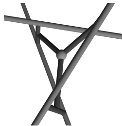
Figure 3: 3D-markers are generated by intersecting rays shot from camera origins through the corresponding image planes into the scene.
