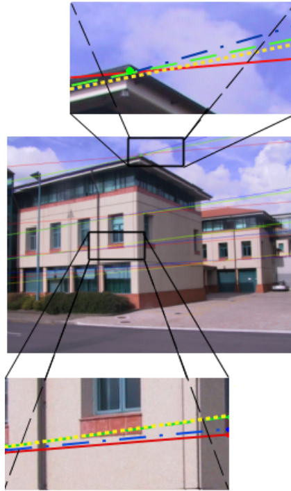
Fig. 5. Epipolar lines result from different data sets. The green lines (dash lines) from data without generated noise; the red lines (straight lines) are from noisy data; the blue lines (dash-dot lines) and yellow lines (dot lines) are from noisy data which has been optimized with collinearity and coplanarity knowledge, respectively.
