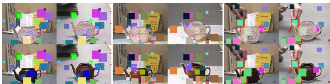
Figure 13. The sequence from Fig. 12 has been disturbed with rectangles of random size, position, and color, which leads to occlusions of the object. Top row: Pose results for different frames. Bottom row: Segmentation results. The occlusions can be compensated due to the object model. The result on the right shows the worst pose according to the diagram in Fig. 12.
