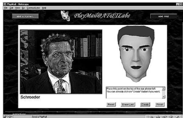
Fig. 24. The user marks feature points in the face manually in order to create a face model. Dots marked in the right, generic face model (see right upper eyelid) guide this process. [Reproduced with permission from J. Ostermann, “E-COAGENT: An electronic convincing agent,” in MPEG-4 Facial Animation: The Standard, Implementation and Applications , I. S. Pandzic and R. Forchheimer, Eds. (Chichester, U.K.: Wiley, 2002) [61]].
