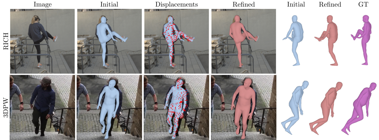
Figure 4. Qualitative results on RICH [19] and 3DPW [61]. From left to right: input images, initial body estimates, our predicted displacement fields, our refined 3D human models and side views of initial, refined and ground-truth bodies.
