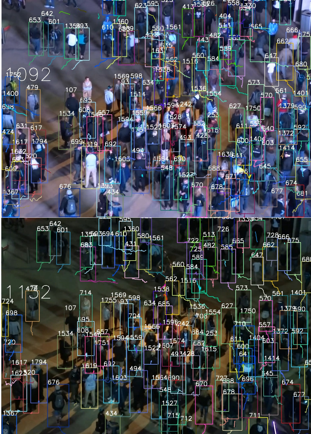
Figure 4. Example images from sequence MOT20-04 at frames 1092 and 1132. The images shows a crowded scene captured by a static camera. The above image is captured before an illumination change happens. The lower image is captured after an illumination change happens. The appearance of persons changes consequently to the illumination changes (e.g. ID 666 in the top right corner). The result video can be found at https://motchallenge.net/method/MOT=4031&chl=13&vidSeq=MOT20-04 .
