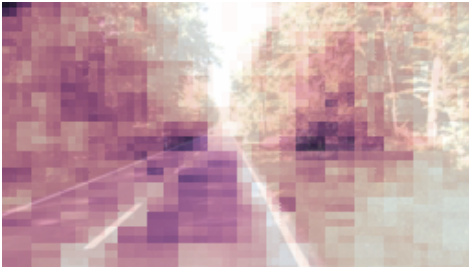
Fig. 3: Usage of the artificial reference picture generated by the neural network trained to optimize the SATD in VTM as a heat map. Linearly scaled from no usage (white) to highest usage (purple).
