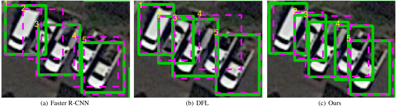
Figure 8. Example images showing the differences between the bounding box predicted by RPN (dashed purple box) and the finally predicted location (solid green box) regressed by the classification layer.
