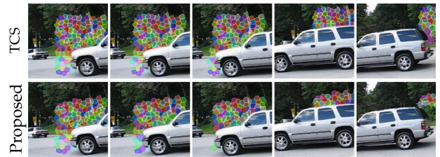
Fig. 13. Qualitative label consistency comparison with [24] on a sequence from [45]. In front of the car, the newly proposed approach correctly deletes the superpixels which should disappear due to the occlusion. Behind the car, new superpixels are created (not displayed) which prevent the superpixels from slipping down.
