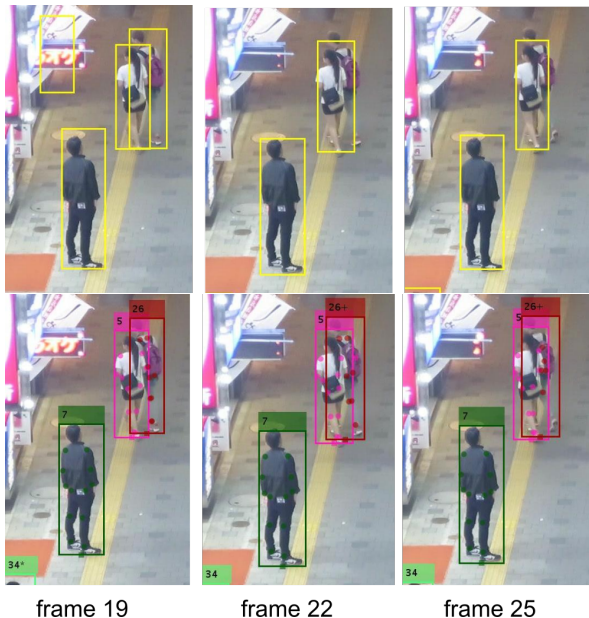
Figure 1. Tracking based on people and joint detections. Top row: SDP input detections on MOT17-04. The person with the red bag is not detected anymore after frame 19. Bottom row: The result of our method. Due to the integration of joint detections into the data association, all persons are found and tracked correctly, despite heavy occlusions and missing detections.
