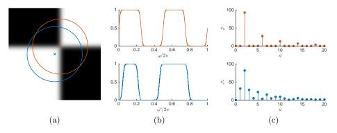
**Fig. 1.** (a) Decentered and blurred x-corner, (b) signal intensities along local polar angles  $\varphi$  (red) and  $\varphi^*$  (blue), and (c) corresponding magnitudes  $c_n$  and  $c_n^*$  of complex Fourier series coefficients.
