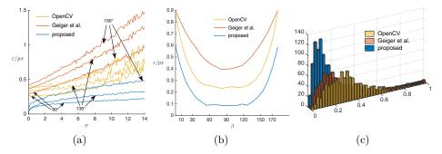
**Fig. 2.** Synthetic x-corners: Absolute localization error (a) w.r.t. blur parameter  $\sigma$ , and (b) w.r.t. distortion angle  $\beta$  at a typical blur level of  $\sigma = 6 \text{ px.}$  (c) Real images: Distribution of reprojection errors  $e_{\text{repr}}$  after camera calibration.
