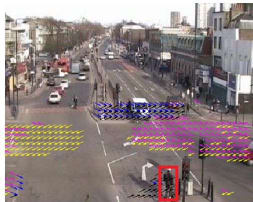
(b) Pedestrian walking in improper area
