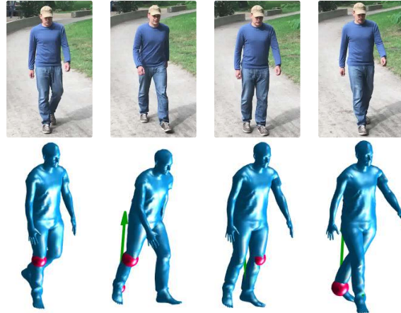
Figure 9. Regression results for an asymmetric gait reconstructed from IMU data [22]. We are able to infer plausible controls despite the higher imprecision of reconstructed model states (e.g. the exaggerated forward bend in the second frame).
