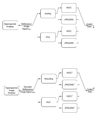
Figure 1. Experimental Setup
