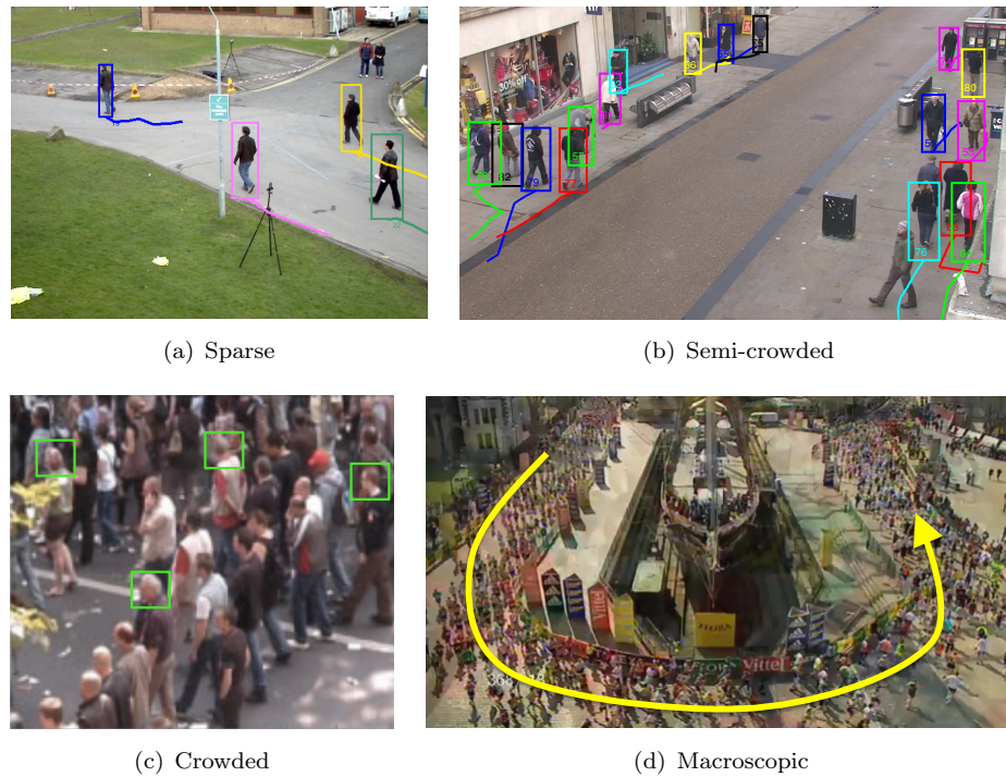
FIGURE 2.1: Scenarios with different crowdness levels. (a) Sparse: individuals are detected and tracked throughout the scene. (b) Semi-crowded: it is still possible to detect individuals, but occlusions and missed detections are very common, making tracking challenging. (c) Crowded: tracking full-body pedestrians is no longer possible, but detection and tracking of heads is still performed. Person counting is a common task for videos of this crowdness level. Image from [Rodriguez et al., 2011a]. (d) Macroscopic scenario: individuals cannot be properly detected, therefore the goal in these scenarios is typically to find the overall flow of the crowd. Image from [Ali and Shah, 2008].
