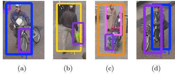
FIGURE 2.9: Example of pedestrians walking with objects. This often leads to double detections or missed detections, but pedestrian-object interactions can be a useful source of information to improve tracking.
