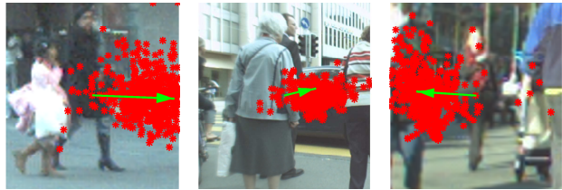
Figure 3: The green arrow indicates the ground truth velocity of the pedestrian, and in red we plot the votes made by the corresponding leaves of the learned RF.
