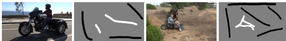
Fig. 2. Example user strokes for the sequences harley and gokart with the original video frames. Foreground is marked white and background black. Only for one frame per sequence user strokes were generated.
