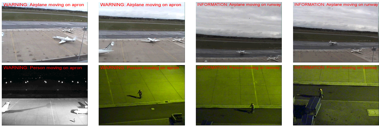
Figure 6: Airplane tracking on apron and runway (top), person tracking on apron and taxiway (bottom). Different messages describing each situation in terms of object, area and danger level are shown. Moreover, in the first sequence a still object is not detected, while the second sequence shows the system robustness to low illumination.
