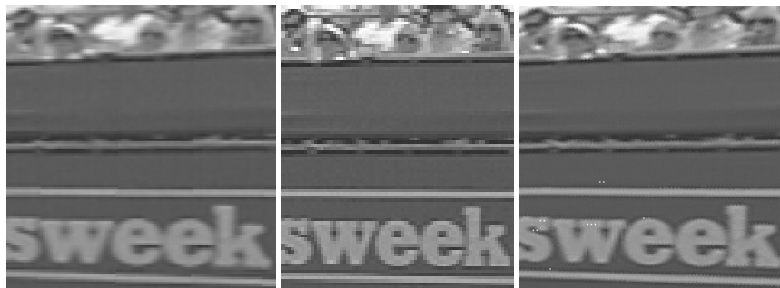
Fig. 3. Left: detail from a conventionally generated mosaic, middle: detail from an original frame, right: detail from a super-resolution mosaic
