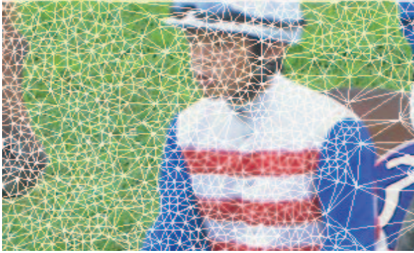
Fig. 2. Triangle mesh for the upper left corner of frame 6 of the RaceHorses sequence.
