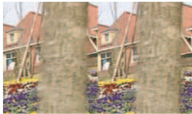
Fig. 7. Interpolation at object borders. Flowergarden sequence, mesh-based on the left, block-based on the right.
