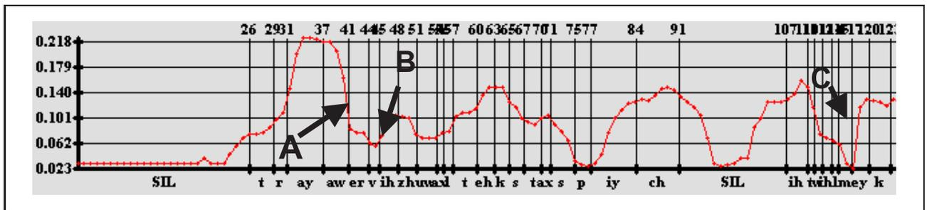
Figure 5. Mouth height as a function of time for the sentence: "Try our Visual Text-to-Speech, it will make ..."; The arrows show where the automatic quality evaluation flagged errors: A: closure too fast; B: missed closure; C: opening too fast. The average contiguous segment length is 6.05 frames with a variance of 2.4 frames, a value judged as good (main influence on 'smoothness').
