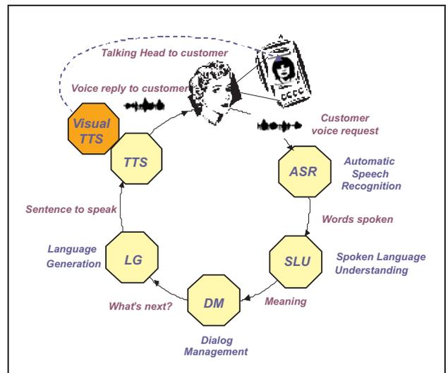
Figure 1. Diagram of any voice-enabled service, extended by Visual Text-to-Speech (VTTS).
