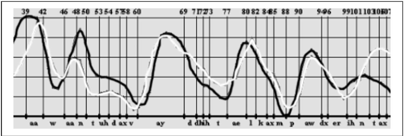
Figure 3. Mouth height as a function of time for the sentence: "I want to divide the talcum powder into ...". The black line shows the recorded values, the white one the values of the synthesized articulation. For a quality score of 'precision', the differences in mouth height between recorded and synthetic samples are summed and normalized by the number of frames.
