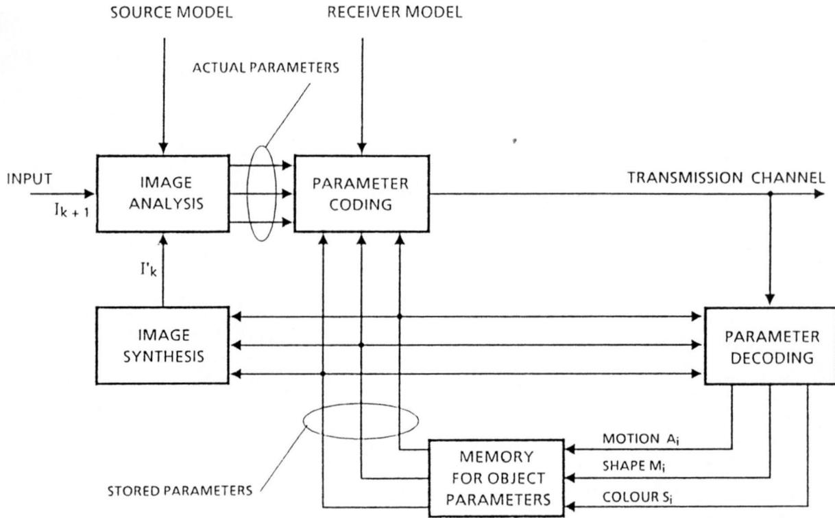
Fig. 1. Block diagram of an object-oriented analysis-synthesis coder
